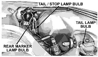
3. Reinstall the appropriate bulb and socket assembly. Replace the access panel. Close the trunk.
